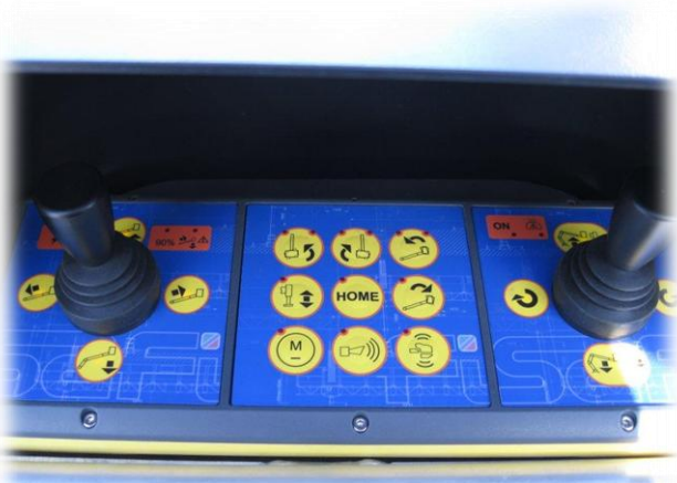
MOBA MULTI PURPOSE CONTROLS - 3 MOVEMENT AT THE SAME TIME
