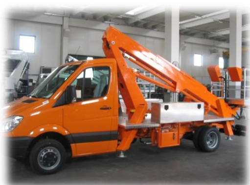
A+A STABILIZERS ON MERCEDES SPRINTER
